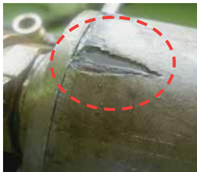
Fig. 2 ESP Casing Corrosion Recovery by Cold Welding
