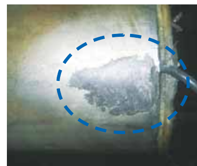
Fig. 2 ESP Casing Corrosion Recovery by Cold Welding
